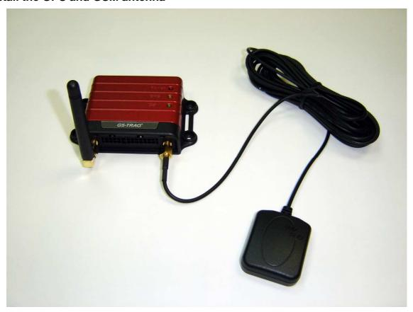
Install the GSM antenna to the GSM antenna port on the left side of the back of the device and install the GPS antenna to the GPS antenna port on the right side of the back of the device making sure both antennas tightly screwed in place. Please refer to the photo above.
