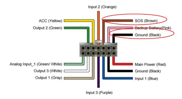
One end of the button must be connected to the SOS line and the other end must be connected to the ground line.
