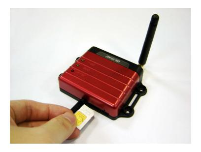
With the cooper contacts face-up, align the notch on the SIM card with the notch on the SIM slot and insert the SIM card. If SIM is inserted correctly, you will not be able to see the copper contacts after inserting the card. To eject SIM card, simply, use your finger nail and apply slight pressure.
