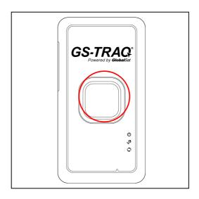
Shortly press the emergency button to make TR-203 connect to Free Web Service.
