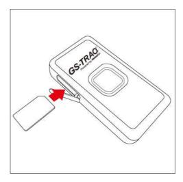
With the metal contacts facedown and the notch on the SIM card left side, insert the SIM card into the SIM holder.
