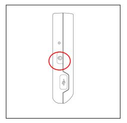
To turn the device "ON", press and hold the power button until you feel the device vibrating.
