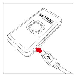
First time users, rechargeable battery requires a complete charge before using TR-203 device.
